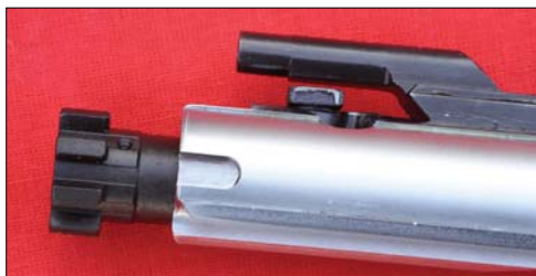
The left-side side charging handle interfaces with a U-shaped notch machined into the left side of the bolt carrier and permits the bolt group to be retracted.
