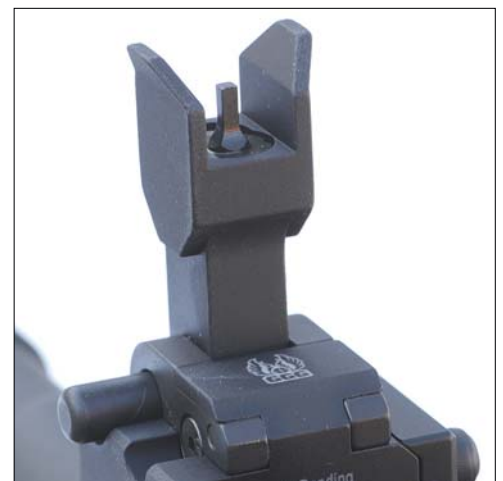
Pushing the actuator button of the GG&G Spring-Actuated Flip-Up Front Sight releases this square-post sight and it pops up to a locked position for instant deployment.
